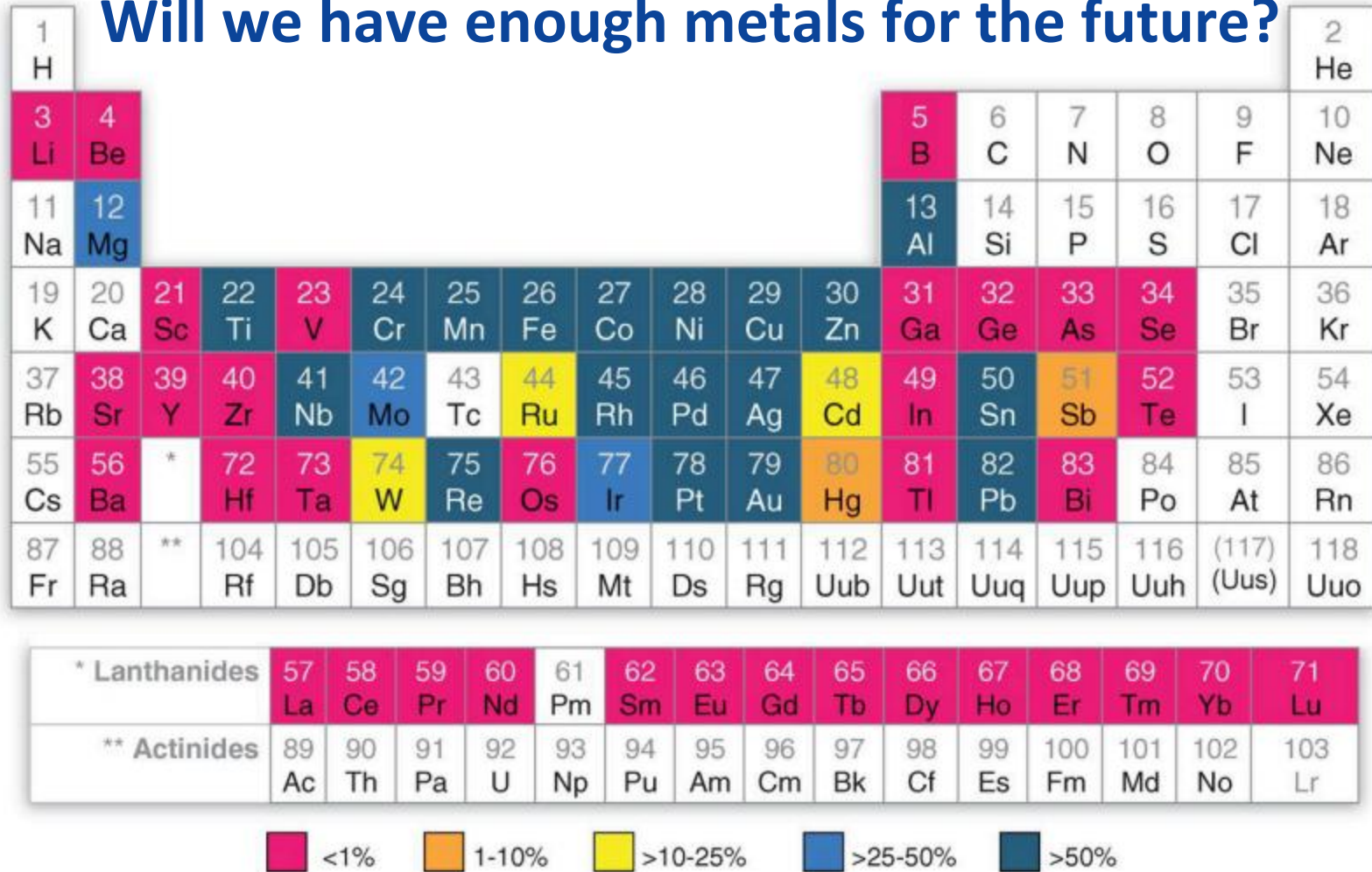
Figure 9.6 Global estimates of end-of-life recycling rates for 60 metals and metalloids: 30 are <1%; 2 are 1-10%; 3 are 10-25%; 3 are 25-50%; only 18 are over 50% (Reck and Graedel 2012, adapted from a figure in Graedel et al. 2011; ©AAAS, reprinted with permission).
