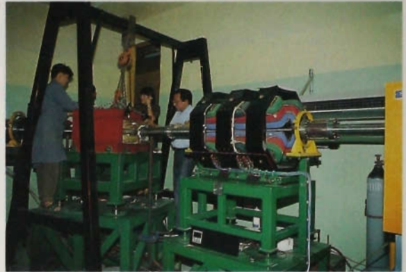
Nitrogen ion implantation system developed by Chiang Mai University with MTEC's support.
