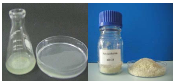
Fig. 2. EPs produced by Nostoc sp. in liquid form (left) and dried form (right)
