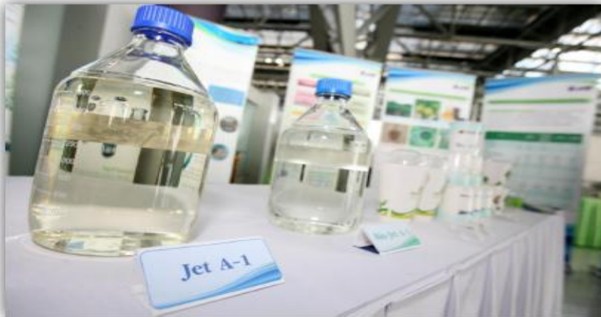
Jet A-1 containing 50% HRJ Fuel certified by ASTM D7566
