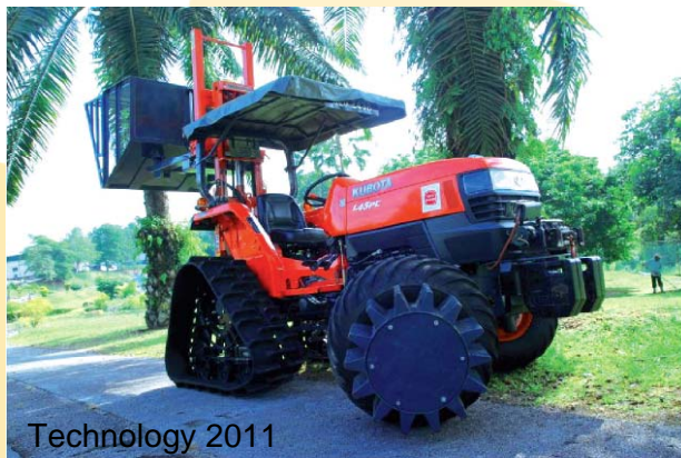
Figure 3. Crawler tractor with a 500-kg forklift bucket.
