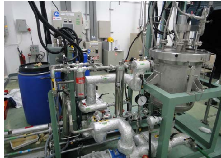
BDF Upgrading Unit (partial hydrogenation of polyunsaturated FAME)
