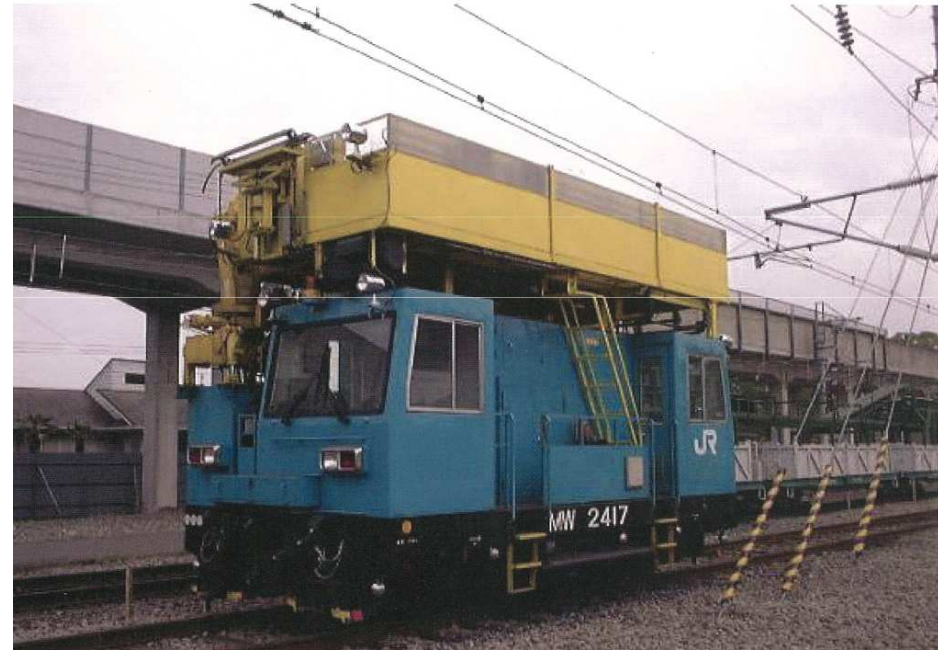
Maintenance Wagon for Overhead Catenary System
