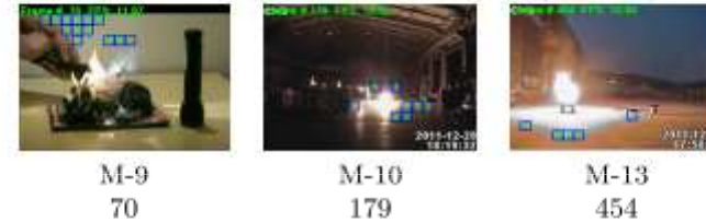
Fig. 11 The first frame in which fire incidents were detected in nighttime video sequences M9, M10, and M13. QuickBlaze detected flame regions, while VisiFire detected smoke regions. Note the better localization of the fire by the proposed method.
