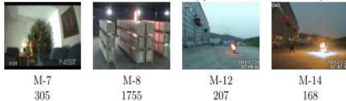
First frame in which fire is detected (VisiFire)
