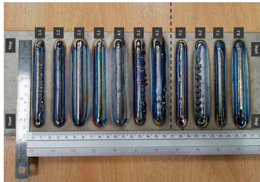
Figure 2. Deposited single beads for a designed experiment for the hot-wire plasma welding process (Numbers 1–8).
