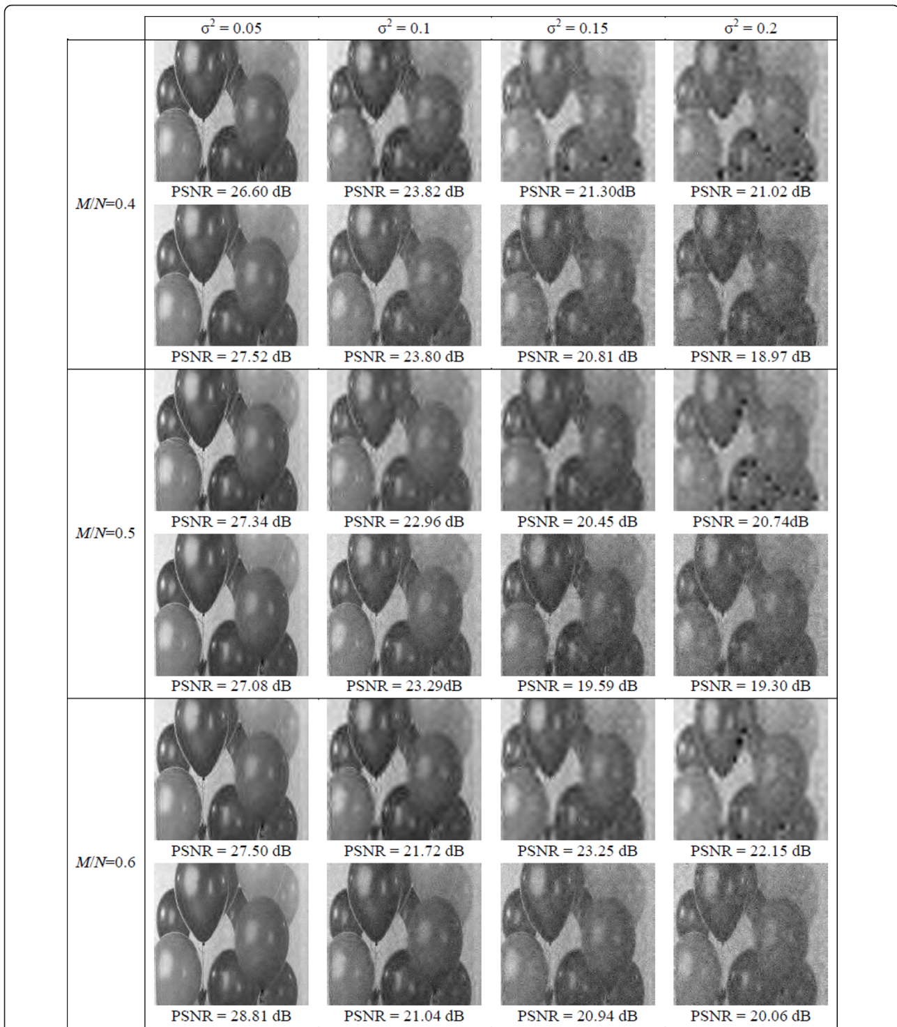
Figure 10 Comparisons of the reconstructed Pallons by DCS-SOMP (top row) and OMP-PKS+RS (bottom row) with M/N = 0.4, 0.5 and 0.6 at \sigma^2 = 0.05, 0.1, 0.15 and 0.2 .
