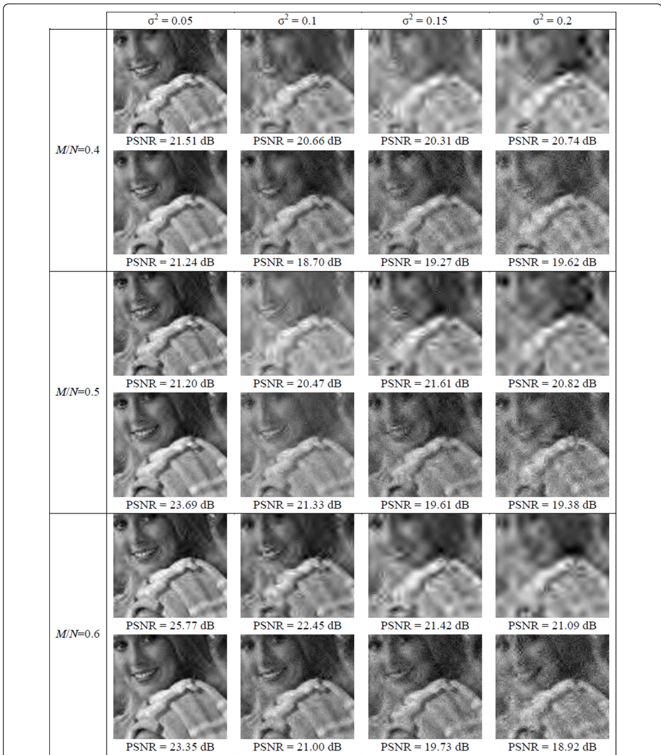
Figure 11 Comparisons of the reconstructed Elaine by DCS-SOMP (top row) and OMP-PKS+RS (bottom row) with M/N = 0.4, 0.5 and 0.6 at \sigma^2 = 0.05, 0.1, 0.15 and 0.2 .
