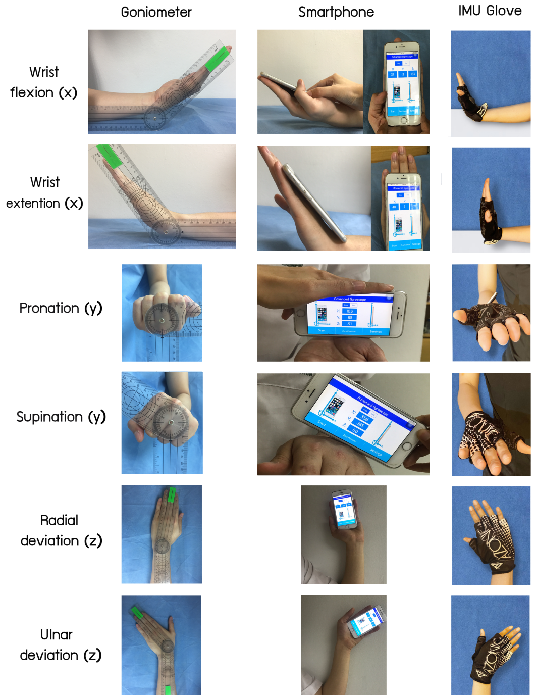
Figure 1. The measurements of wrist range of motion using a standard goniometer, smartphone, and the proposed inertial measurement unit glove for wrist flexion (x), wrist extension (x), pronation (y), supination (y), radial deviation (z), and ulnar deviation (z).
